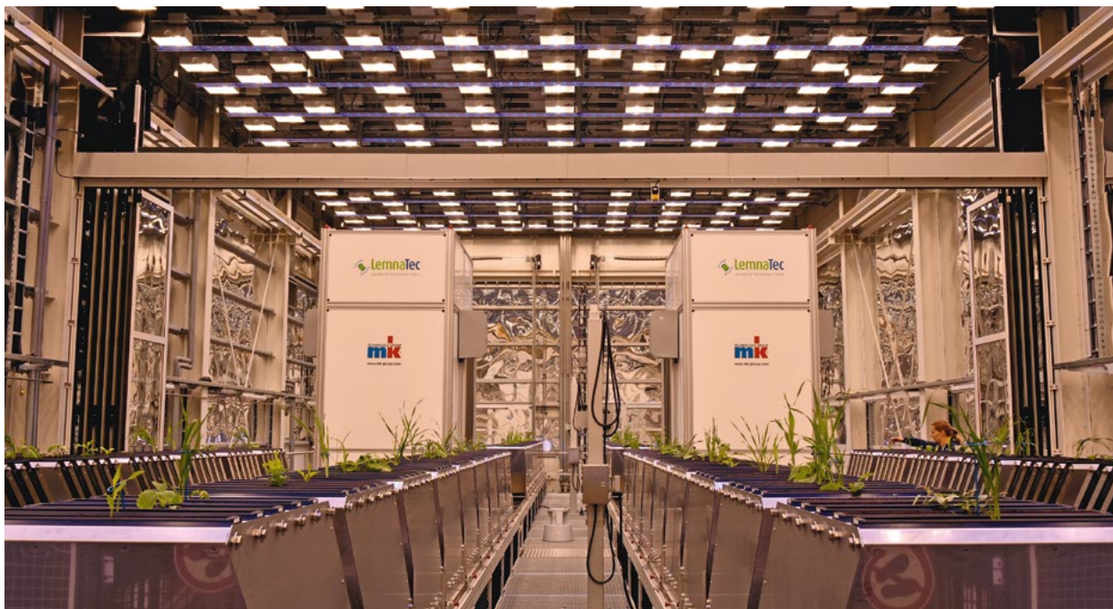
Rhizotron system in the PhenoSphere for automated digital phenotyping of above- and below-ground plant parts.
